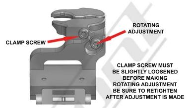
**STEP 5 -** Use adjustments shown to install RD to your desired position. We recommend adjusting RD as close to bottom of mirror as possible. Be sure to tighten vertical and pivot adjustment screws after adjustments are made. For Pivot adjustment, grab long arm of allen wrench for maximum leverage. You will not strip the threaded holes in the aircraft grade aluminum.
