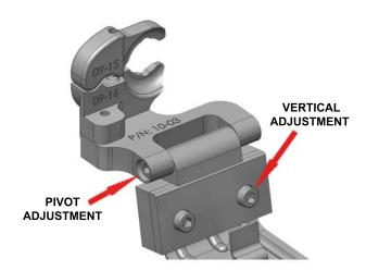
**STEP 4** - When the mount is positioned as far forrward as it will go, tighten the clamp screw untill the Top and Mid Sections are **slightly snug** around the mirror stem. You should still be able to rotate the mount. Rotate the mount so it is parallel with the bottom of the mirror. Tighten the clamp screw untill the mount is securely attached to the mirror stem.
