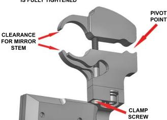
STEP 3 - BEFORE FULLY TIGHTENING THE CLAMP SCREW, POSITION THE MOUNT AS FAR FORWARD TOWARDS THE WINDSHIELD AS YOU CAN. MAKE SURE THE TOP AND MID SECTIONS ARE TOUCHING AT THE PIVOT POINT. If you can not get them to touch at the pivot point, you have an incompatible mirror type for this mount.
